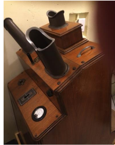
X-Ray unit in storage, used in mid-20 th century stores to fit customers for shoes. Photo credit: Kristen Vogt Veggeberg.
