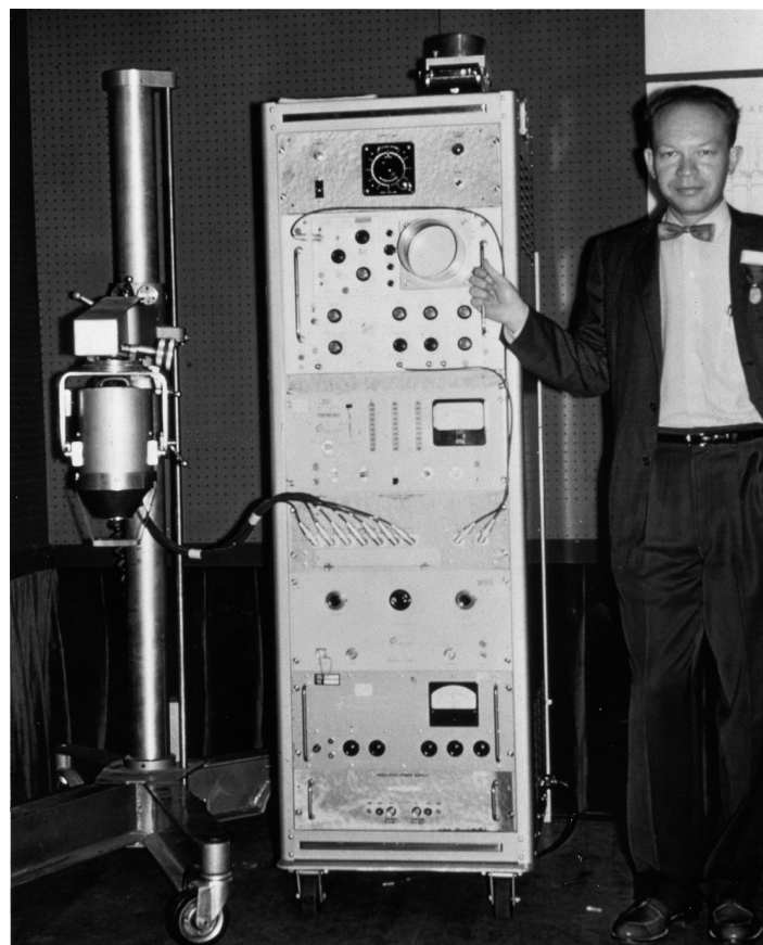
Figure 4: Hal O. Anger with an early version of the Anger scintillation camera, also called a gamma camera. (Photograph from the Myers Collection)
